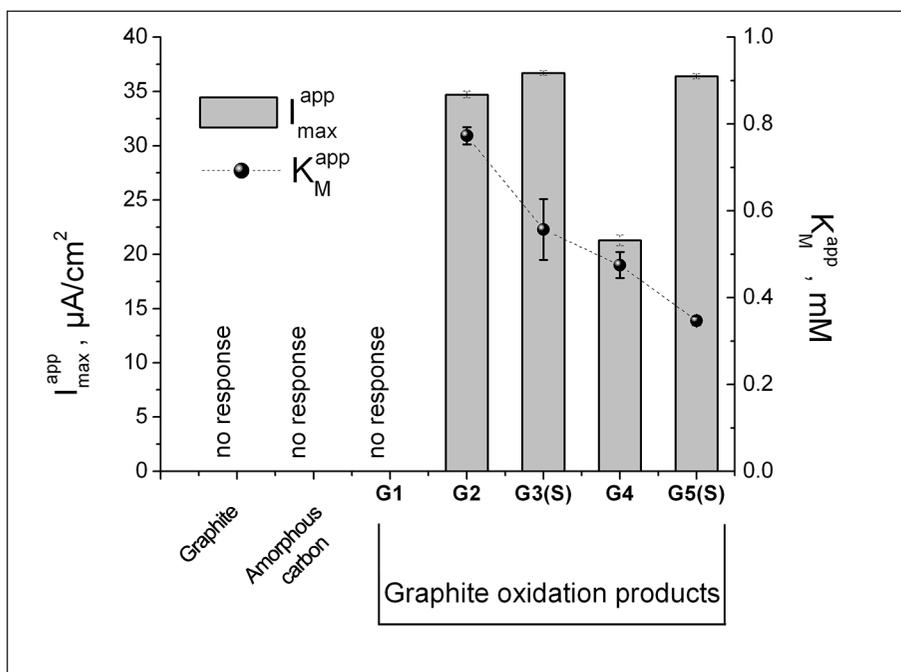
**Fig. 4.** Kinetic characteristics of bioelectrocatalytic systems with PQQ-GDH and CME materials
