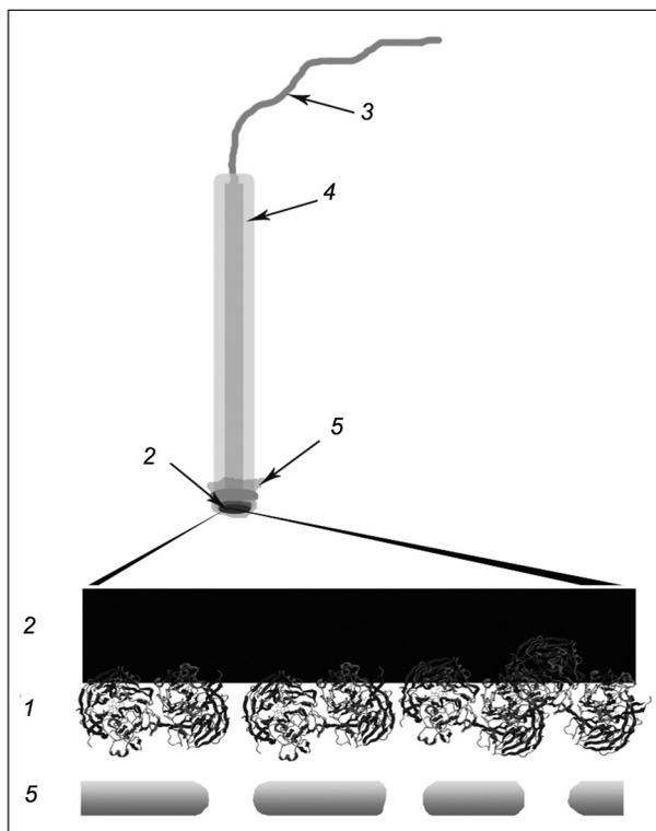
**Fig. 2.** Scheme of construction of bioelectrocatalytic system based on enzyme and CME. 1 – layer of enzyme, 2 – CME surface, 3 – CME contact area, 4 – insulating layer, 5 – protective semipermeable membrane
