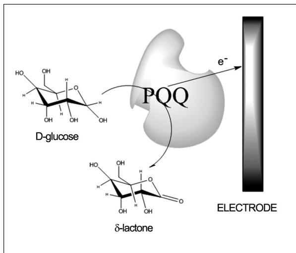
**Fig. 3.** Proposed mechanism of DET in bioelectrocatalytic systems with PQQ-GDH
