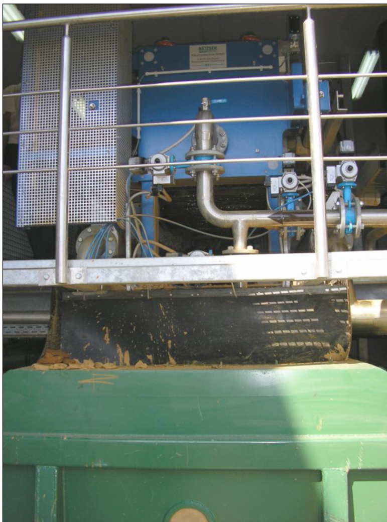
Fig. 2. Press-filter producing pressed backwash residual cake (Antaviliai, Lithuania)
