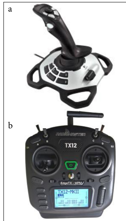
Fig. 2. External appearance of the joysticks used in the experimental study: a – Logitech Extreme 3D Pro L942-000031; b – Radiomaster TX12
