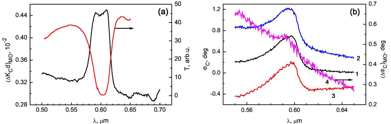
Fig. 5. (a) MCD, transmission  $T$ , and (b) Faraday rotation spectra of sample OP11 of Co-modified opal crystal immersed in isopropyl alcohol. In (b) the spectra are shown for magnetic field 0 (1), +350 mT (2), -350 mT (3), and resulting MO effect (4).
