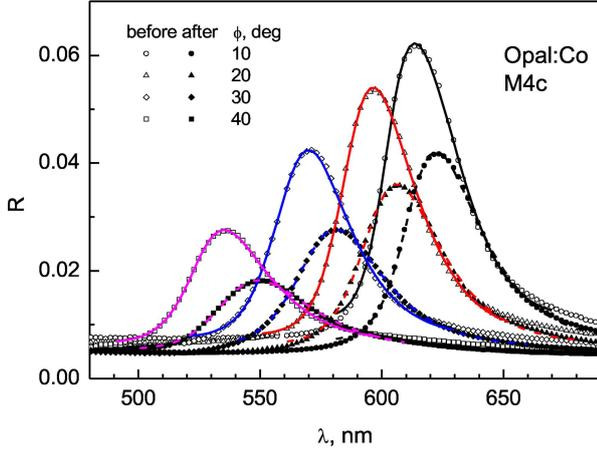
Fig. 4. Experimental (points) reflection spectra approximated by asymmetric lines (curves) at various angles of light incidence for opal crystal (sample M4c) before and after formation of Co nanoparticles inside opal lattice.
