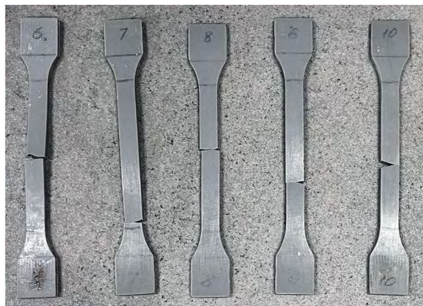
Fig. 4. The tensile tested Phrozen Aqua 8K Series Resin samples (marked from 6 to 10 left to right).
