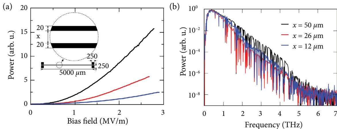
Fig. 1. A photoconductive switch with a coplanar stripline contact geometry (insert) operates at varying gap widths labelled as  $x$ . (a) shows the emitted THz power at different bias fields, while (b) presents the detected spectra using a *TeraVil* THz time-domain spectroscopy setup [15]. In both cases, the switches are photoexcited at  $20 \mu\text{J}/\text{cm}^2$  fluence.
