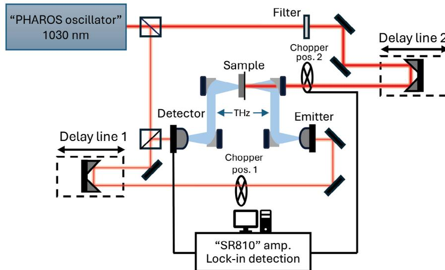
Fig. 1. Experimental setup of the optical pump–THz probe measurement. Chopper position was changed through the experiment. For setup calibration, the chopper was kept in the emitter branch (position 1) to set the required delay after which it was moved to position 2 to measure the pump–probe kinetics.
