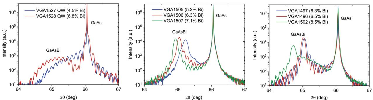
Fig. 2.  $\omega$ - $2\theta$  diffraction scans of (004) plane. GaAs substrate and GaAsBi peaks are named accordingly. The exact Bi content of the sample was evaluated by fitting the XRD results as displayed in the graph legends.
